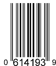
Figure 5-13 Example of UPC-E symbol
