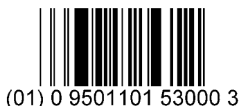
Figure 5-18 Example of GS1 DataBar omnidirectional symbol
