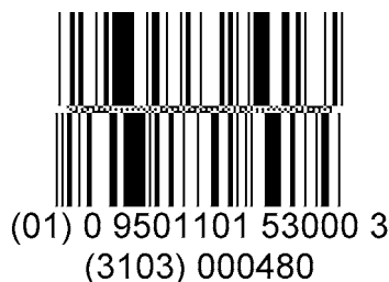
Figure 5-20 Example of GS1 DataBar expanded stacked symbol
