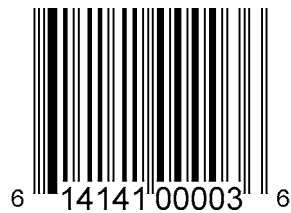
Figure 5-12 Example of UPC-A symbol
