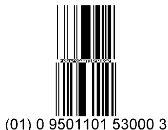
Figure 5-19 Example of GS1 DataBar stacked omnidirectional symbol
